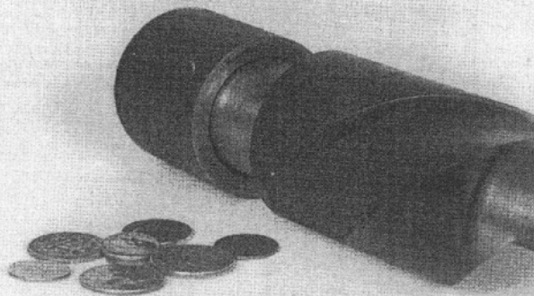
Figure 10 Running Clearance Increase Caused By Very Fine Contaminant
